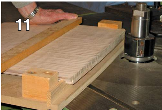
Shaper doing bottom edge—shows bottom panel slot for positioning on jig
