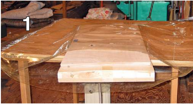
One of the curved side panels exiting the vacuum bag
