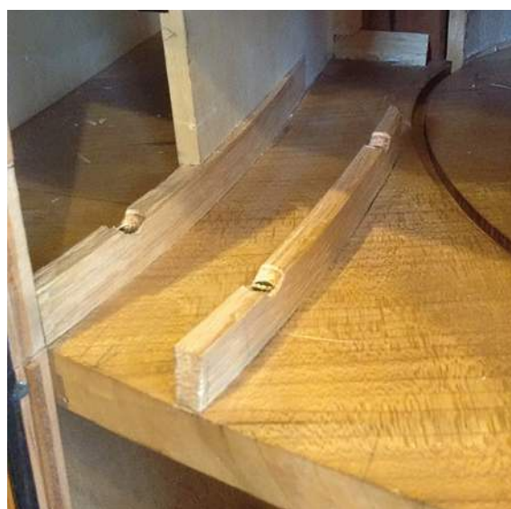
Tight tolerances, with one guide let into the internal divider (on left) and a tambour door sliding by on the right
