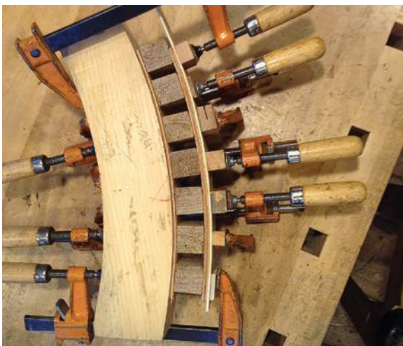
Laminating the two sides with blocks the width of the inside of the drawer separating the two
