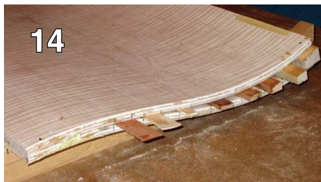
End view of top construction—two 3/8" panels, each of three 1/8" glued up with graduated spacers
