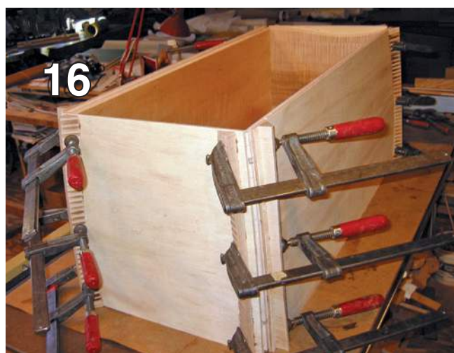
Carcass clamped—note curved 45° clamping ridges glued on wiggly ply
