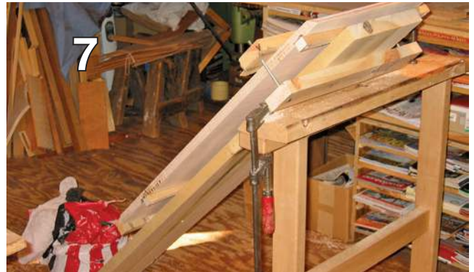
Jig for holding side at 45° for slot
