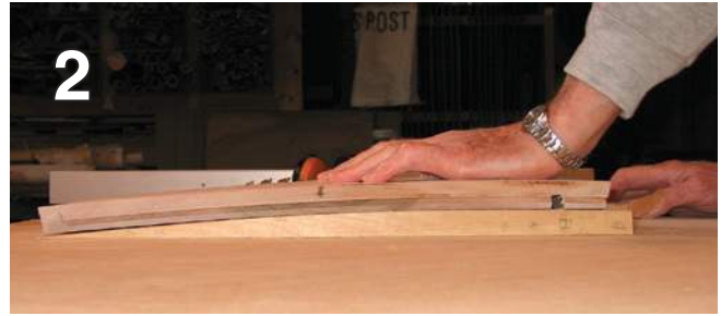
Panel shimmed up to reflect angle on shop drawing
