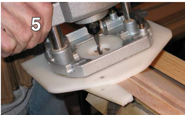
Running the router using the delrin fence on the pointy edge
