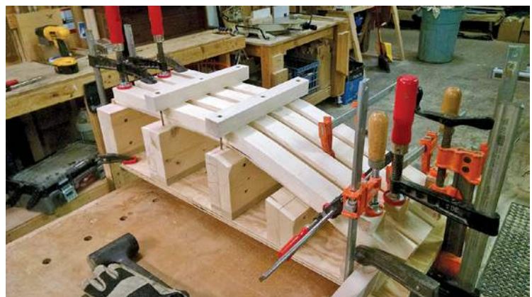
Over-bend form using clamp exchange—set for a day
