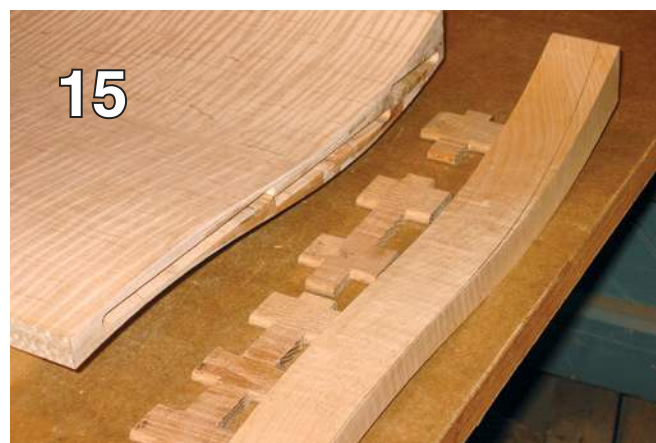
Loose splines for attaching the end batten
