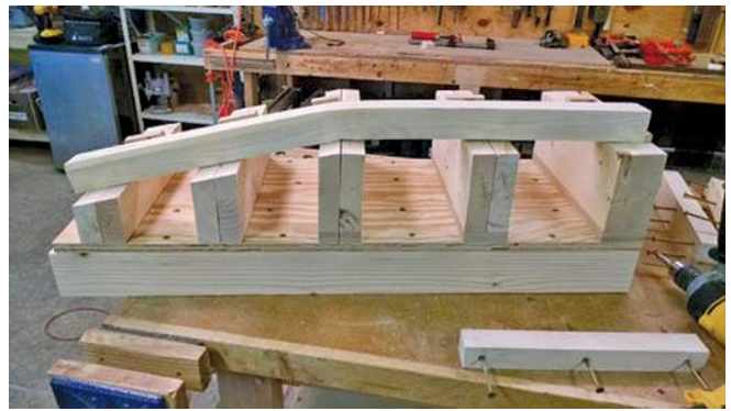
Final form matching spring back and my desired angle
