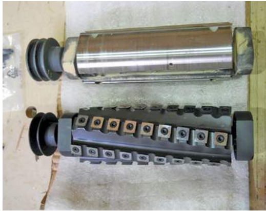
Straight knife cutterhead—top Insert cutterhead—bottom
