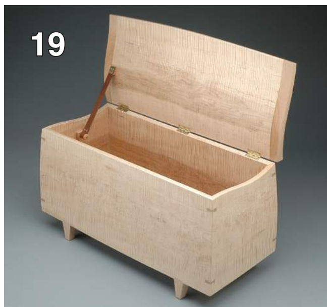
1" wide leather strap restrains the top
