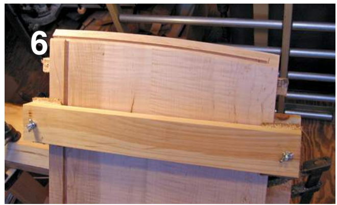
Curved slot at 45°—face with the slot is jugged up to be level
