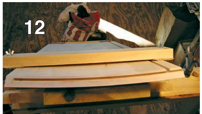
Curved spline slot in 45 joint also shows slot for bottom panel
