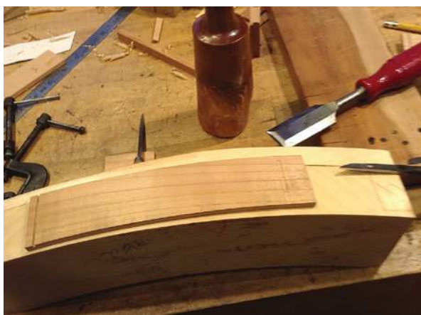
Using the form to support a side while cutting the joinery
