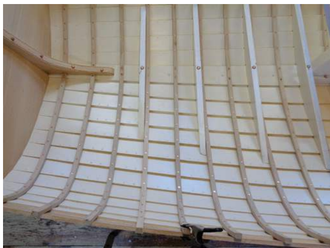
Plenty of rivets to hold everything together
