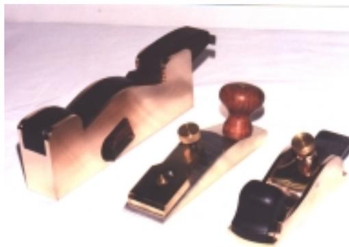
eight pins were press fit into place to mechanically anchor the sole to the plane. The mouth is very tight at 0.018 inches and the blade is bedded at 18 degrees.
